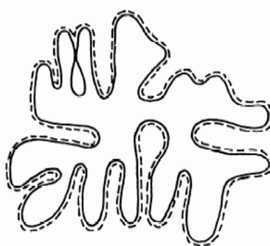
Figure 2 — Schematic cross-section of a particle with surface detected by the adsorption method shown by dotted line
